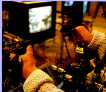
Puppeteer Dave Greenaway at the controls of Raphael, on the video monitor before him, during close-ups filming. In the background Raphael can be seen with off-camera Mark Caso as Leonardo, head off, feeding lines to Raphael's Kenn Troum. Left and Right: The control box, showing Greenaway's hands-on technique. At right is the red "mouth," which swivels right and left. The joystick at left moves in a variety of directions, also with thumb and finger buttons. Behind headset, center, is the unit's LCD display with function buttons.
